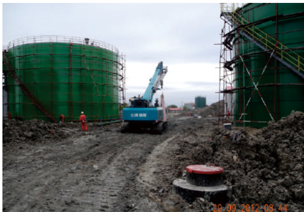
SWTC25在大庆油田工地带载行走作业 SWTC25 Traveling With Load In Daqing Oil Field
